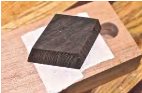
▲ Pic.13 Because the piece was so small, I attached it to a larger board, then ran it through the table saw for the bevel on the edge side
